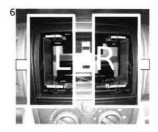
6 These are the brackets mounted inside the radio housing. Pay attention to the letters on the brackets.
