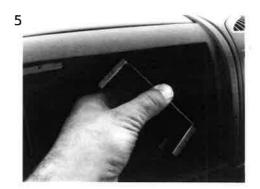
5 Put the mounting brackets inside the radio housing.
