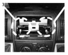
3 Cut and remove the plastic parts. Picture on the left shows the result after cut the plastic frames.
