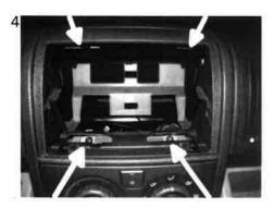
4 Remove the four screws as shown.
